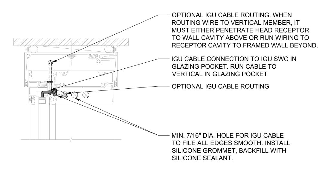
**INSTALLER TO PROVIDE GROMMETS** AT ALL FRAME PENETRATIONS WHERE POSSIBLE TO AVOID CABLE
